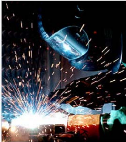
Gas metal arc welding
