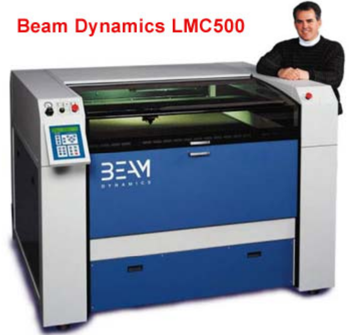
Enclosed Fumes evacuated through ducts
